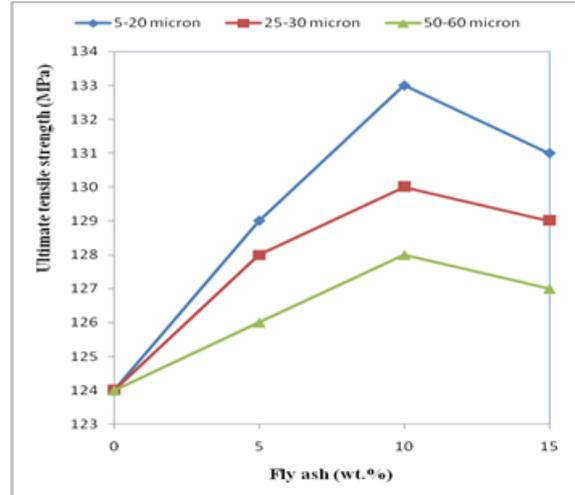
Table3.1 Results of Tensile test carried on various MMCs
