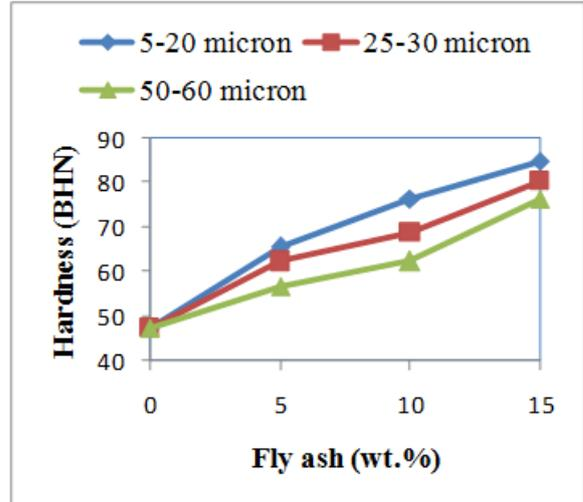
Fig 3.3 Hardness with the wt % of fly ash
