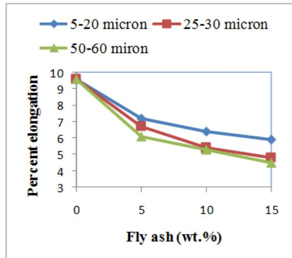
Fig 3.4 Ductility with the wt % of fly ash
